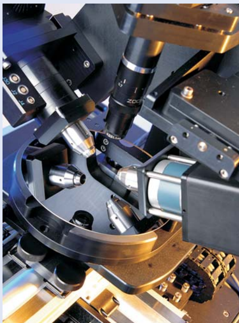
Figure 1. Ellipsometers analyze the reflections of polarized light to determine various material properties. In this photograph, the left arm provides the incoming beam and the right one collects the outgoing light. Both are reflected in the eight-inch-diameter silicon wafer whose properties are being measured. The components described in the text are hidden in the arms. (Courtesy of J. A. Woollam Co Inc.)
